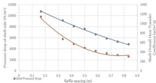
Figure 5 Baffle spacing against shell heat transfer coefficient and shell pressure drop
