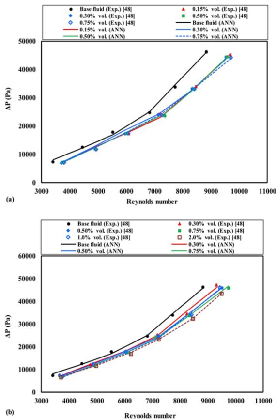
Figure 3 Pressre drop of nanofluid vs Reynolds number
