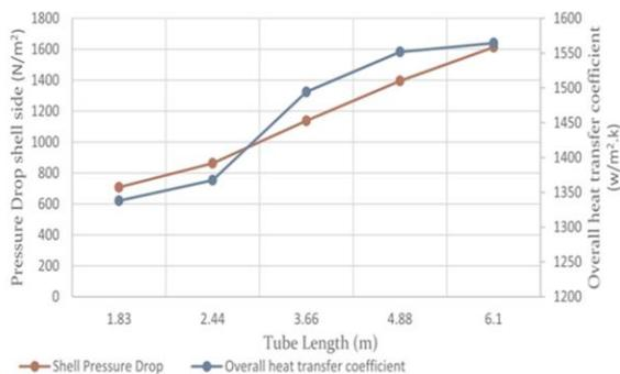
Figure 4 Tube length against heat transfer coefficient and pressure drop for shell drop
