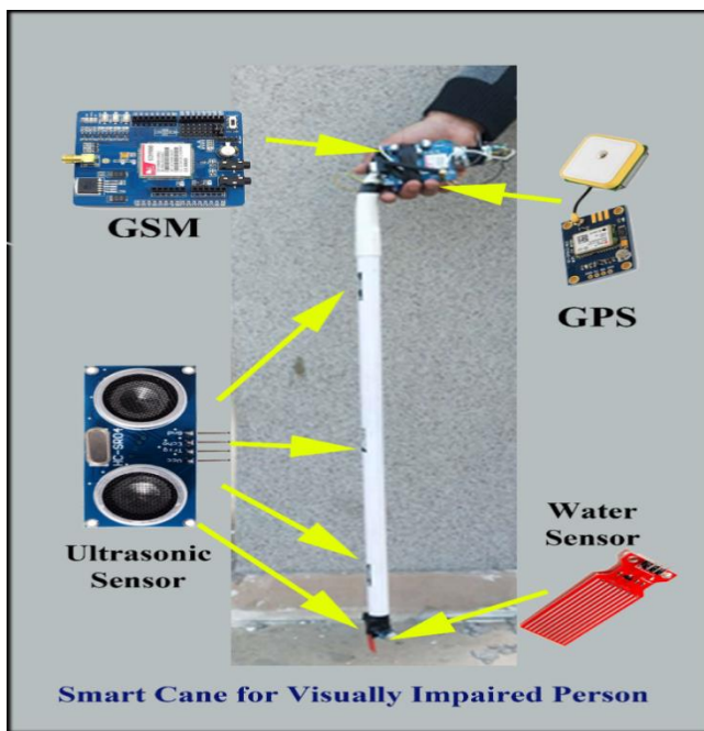
Figure 1: Developed cane equipped with sensors
